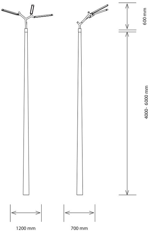
Branch street light is designed to lighten traffic areas and parks. The shape of Branch was inspired by the crown of a pine tree. The elements of the lighting fitting can be freely directed with a joint - this enables to light the road, the surrounding buildings as well as different objects at the same time. The number of LED profiles in the crown of Branch can vary according to the design and goals of the lighting solution.
